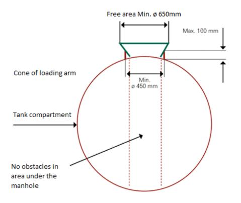
On certain loading bays, namely B01 and B03, Vopak Vlaardingen uses the so-called "cone loading arm". The cone loading arm has to fit exactly when it is lowered into the manhole. It is therefore important that there are no obstacles on the inside of the manhole, such as hooks, couplings, etc. (see photos). If there are obstacles on the inside of the inside of the manhole, then loading cannot take place.
